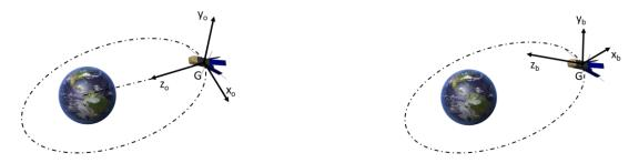
Figure 4. Cartesian Reference Frames. (Left) Orbit Frame (F<sub>0</sub>). (Right) Body Frame (F<sub>b</sub>).
